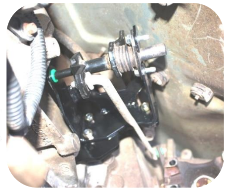
Figure 9 Transfer Case Linkage Installed
